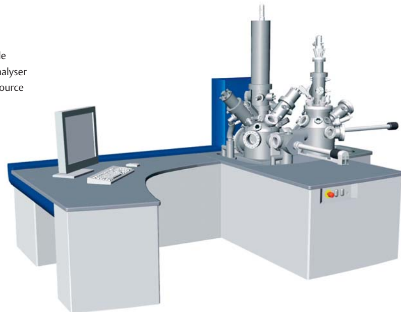
Qtac bolt-on module attached to the preparation chamber of a TOF.SIMS 5
