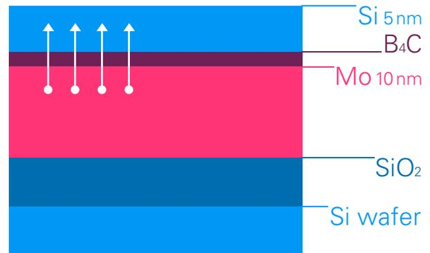
Si/Mo layer structure with an ultra thin B<sub>4</sub>C diffusion barrier
